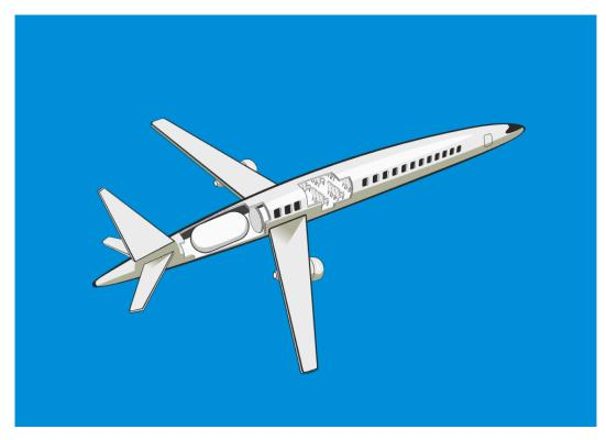
Figure 4. Representation of the tank and passenger cabin layout for the LH<sub>2</sub>-powered narrow-body
