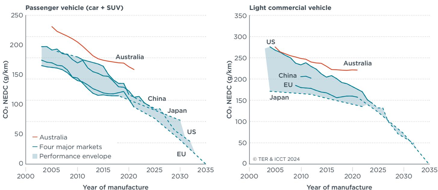
**Figure 2.** Australian LDV (exhaust) tailpipe CO<sub>2</sub> emissions normalized to the NEDC test protocol in an international context; the blue polygon shows the performance envelope with the combined results for China, the European Union, Japan, and the United States. Dotted line = interpolated values or future target values.
