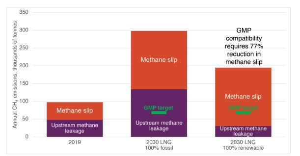
Methane emissions from LNG-fueled ships calling on EU ports in 2019 and two 2030 scenarios compared with the COP26 Global Methane Pledge target of cutting global methane emissions at least 30% by 2030.
