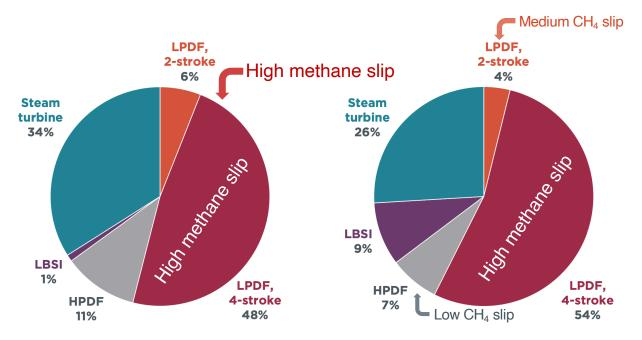
**Figure 5.** LNG fuel consumption by engine type for ships on voyages to, from, and between EU ports in 2019 (left) and predicted for 2030 (right).
