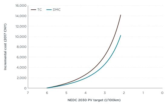
**Figure A2.** 2030 NEDC fuel consumption compliance costs for passenger vehicles under ICE strategy (C Class).
