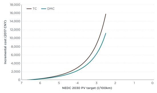
**Figure 4.** 2030 NEDC fuel consumption incremental compliance costs for passenger vehicles under ICE strategy.
