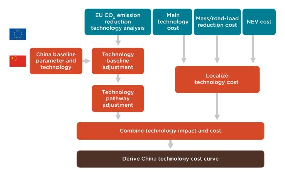
Figure 1. Overview of China technology cost curve methodology.
