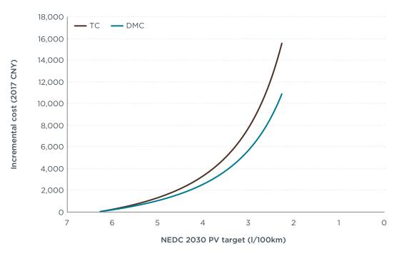
**Figure A3.** 2030 NEDC fuel consumption compliance costs for passenger vehicles under ICE strategy (D Class).
