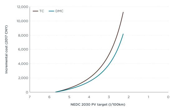
**Figure A1.** 2030 NEDC fuel consumption compliance costs for passenger vehicles (PV) under ICE strategy (B Class).
