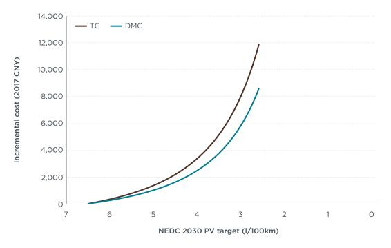
**Figure A6.** 2030 NEDC fuel consumption compliance costs for passenger vehicles under ICE strategy (minivan class).
