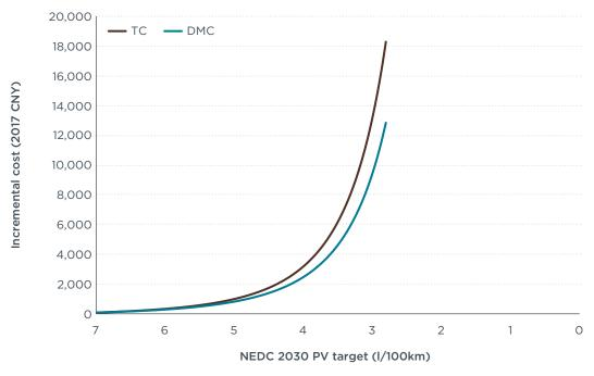
**Figure A4.** 2030 NEDC fuel consumption compliance costs for passenger vehicles under ICE strategy (SUV Class).
